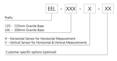
The standard configuration for the EEL is EEL-200-H
